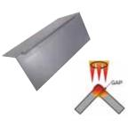
The concentrated heat input in combination with the innovative laser spinning process allows an optimum, consistent welding quality and gap bridging for thin
