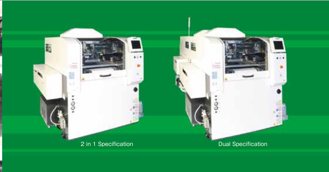
2 in 1 Printing Function Printing both sides of PCB by one machine
